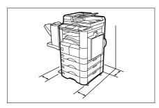
Install the machine on a flat surface, leave at least 4 inches (10 cm) of space between the machine and other objects.
